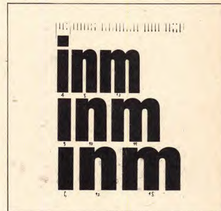
The early Linofilm offered three ranges within which to vary letter widths, an improvement over the restrictions of metal but still very restrictive when compared to more recent machines.
